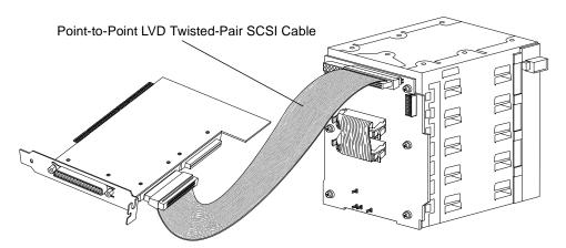
Figure 1-7. Hot-Plug Cage Cable Connections
